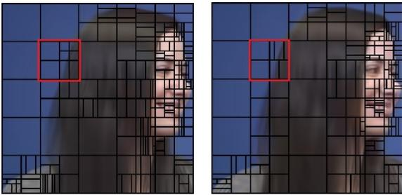
Fig. 8. The CU structure partition result of the default VTM (left) and proposed method (right)
