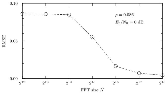
Fig. 6. RMSE of the estimated blockage ratio vs. FFT size characteristics.
