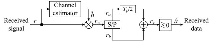
Fig. 2. Configuration of the receiver.
