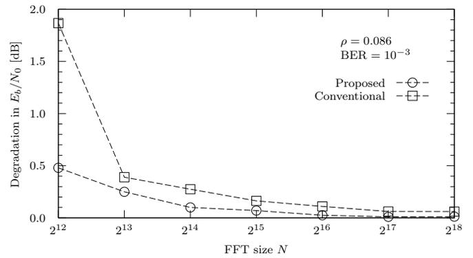
Fig. 8. Dependence of BER performance degradation on FFT size.
