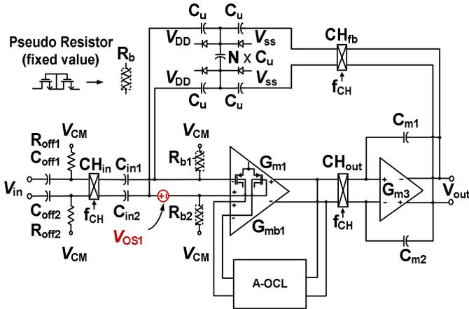
Fig. 2. Schematic of the proposed CCIA using A-OCL.
