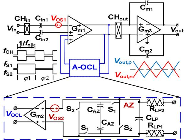
Fig. 3. Schematic of the proposed A-OCL.
