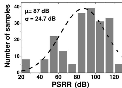
Fig. 10. Monte Carlo simulated PSRR result of CCIA.
