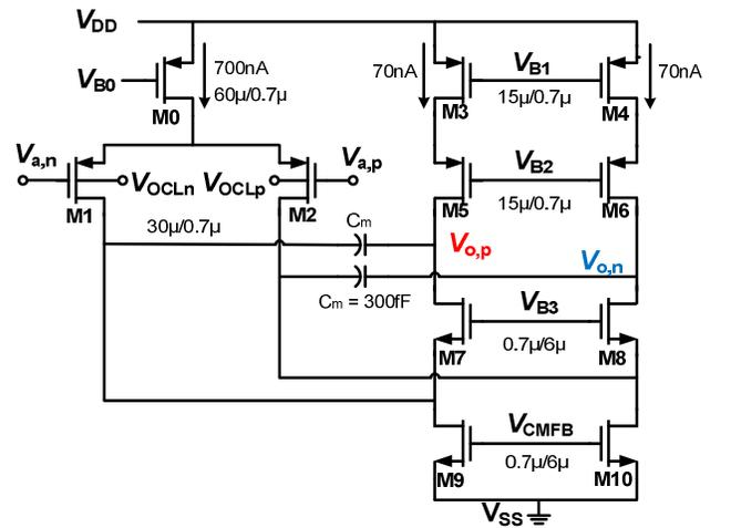
Fig. 4. Schematic of folded-cascode opamp  $G_{m1}$  using buck control input differential pair CMOS transistors.
