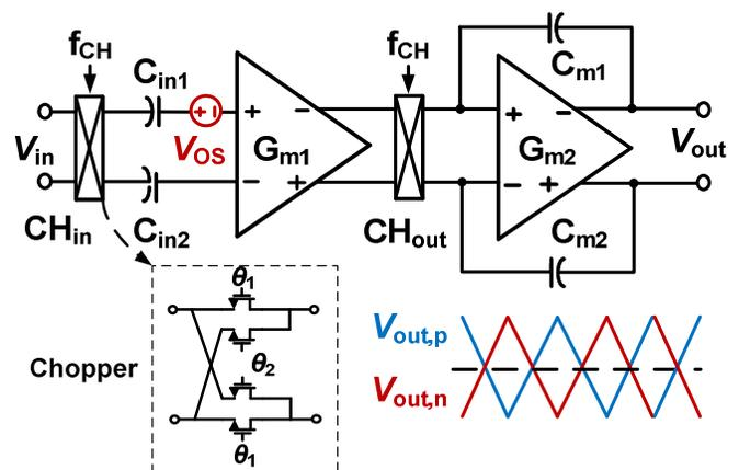
Fig. 1. Schematic of the chopper amplifier.
