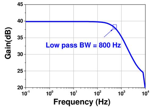
Fig. 9. Simulated frequency response of the proposed CCIA.
