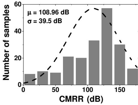
Fig. 11. Monte Carlo simulated CMRR result of CCIA.
