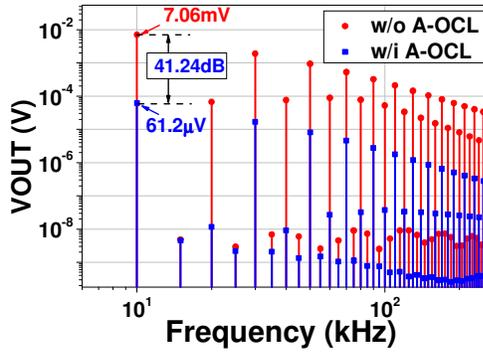
Fig. 12. Spectrum output voltage in cases with and without A-OCL.
