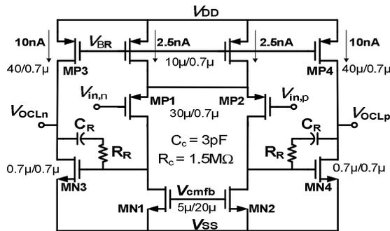
Fig. 6. Schematic of a two-stage opamp  $G_{m2}$  in A-OCL.
