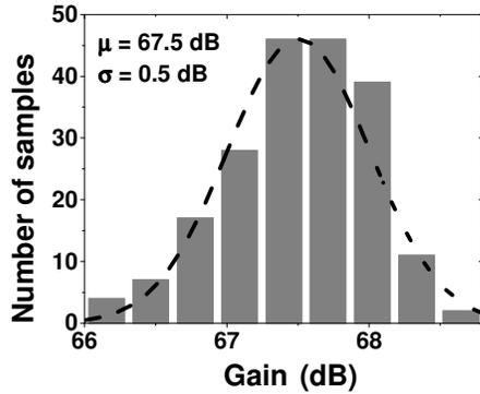
Fig. 5. Statistical distribution of the gain of  $G_{m1}$ .
