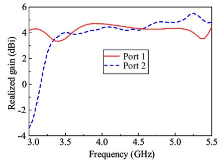
Fig.11. Peak realized gain of the dual-polarized omnidirectional antenna.
