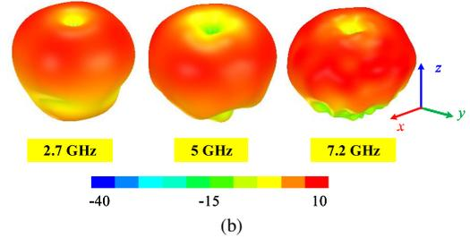
Fig.3. (a)  $|S_{11}|$ ; (b) 3-D total gain radiation patterns of the VP element.
