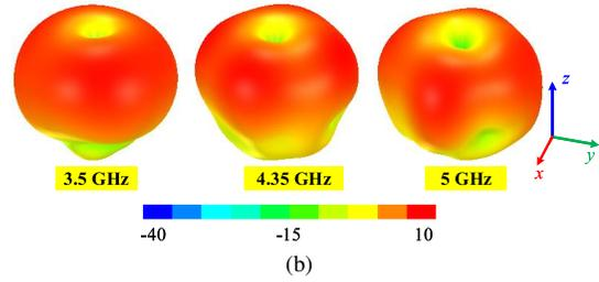
Fig.7. (a)  $|S_{11}|$ ; (b) 3-D total gain radiation pattern of the array dipoles antenna.
