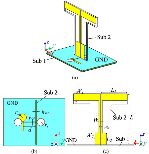
Fig.4. Geometry of the horizontal dipole (a) Perspective view (b) Top view (c) Side view. The design parameters of HP single element are:  $w = 0.8$ ,  $w_1 = 4$ ,  $w_2 = 4$ ,  $w_s = 0.3$ ,  $L = 30$ ,  $L_1 = 15.5$ ,  $L_2 = 9$ ,  $w_d = 0.2$ ,  $w_{ms} = 1.1$ ,  $R_s = 1.8$ ,  $R_m = 1.8$ ,  $d = 9$ .
