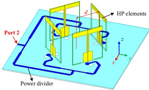
Fig.6. Geometry of the dipoles array antenna.
