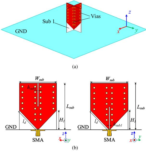
Fig.2. Geometry of the VP element: (a) Perspective view; (b) Front views. The parameters of VP element are  $W_{sub} = 20$ ,  $L_{sub} = 25$ ,  $H_1 = 10$ ,  $h_{sub1} = 0.508$ .
