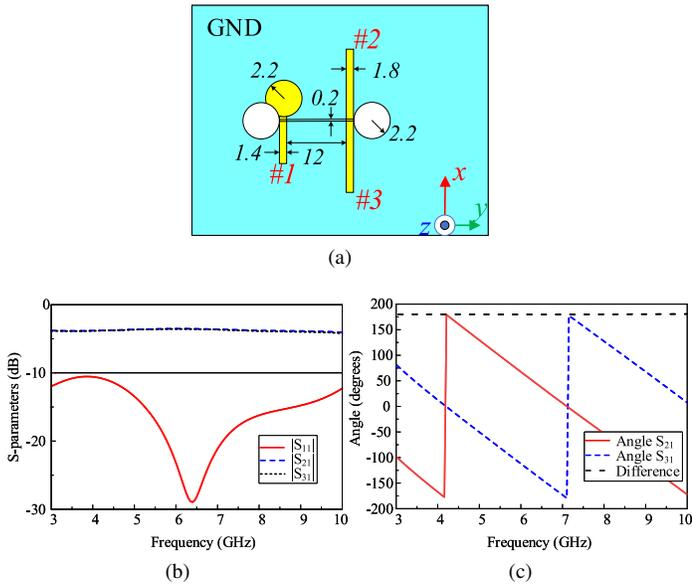
Fig.5. (a) Geometry of the out-of-phase power divider; (b) its S-parameters and (c) Phases.
