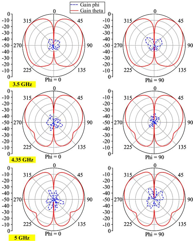
Fig.9. Radiation pattern of the VP element.
