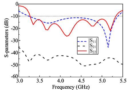
Fig.8. (a) Geometry of the proposed antenna; (b) S-parameters of the design antenna.
