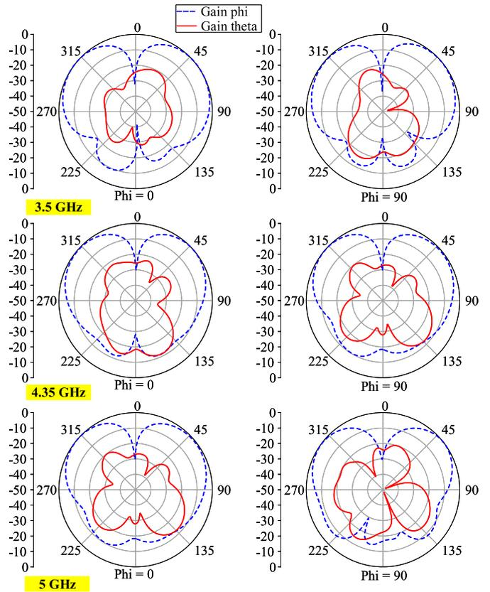
Fig.10. Radiation pattern of the HP element.
