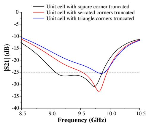
Fig. 3. Simulated input port isolation of proposed antenna with the different corners truncated.
