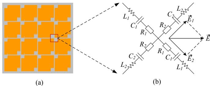
Fig. 1. The spatial equivalent circuit of the metal microstrip structure on the metasurface.
