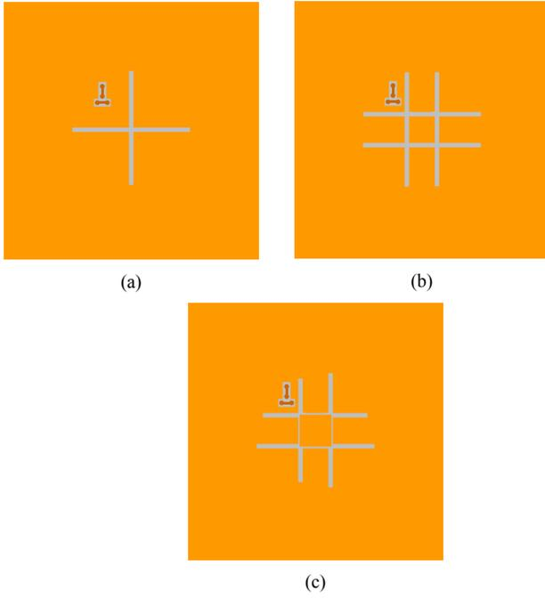
Fig. 4. Ground of proposed antenna with: (a) Cross-slot, (b) # shaped-slot, (c) Unbalanced #-shaped slot.
