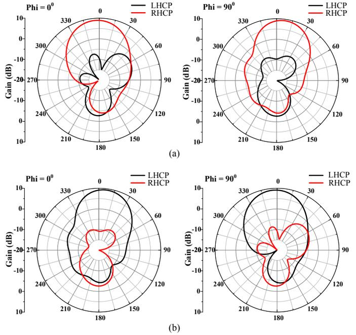
Fig. 10. Simulated radiations and gains of proposed antenna excited by two ports: (a) Port 1, (b) Port 2.
