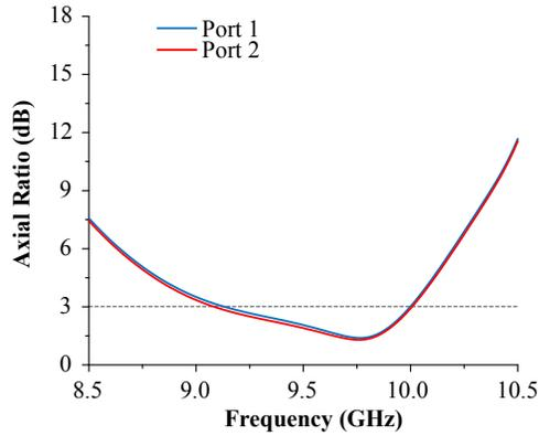
Fig. 8. Simulated axis ratio of proposed antenna
