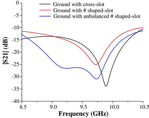
Fig. 5. Simulated input port isolation of proposed antenna with the different grounds.
