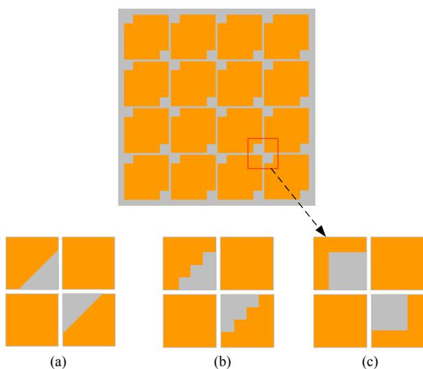
Fig. 2. Unit cell with: (a) triangle corners truncated, (b) serrated corners truncated, (c) square corners truncated.
