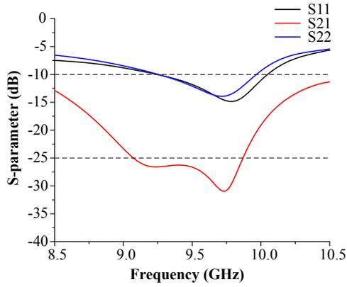
Fig. 7. Simulated S-parameter of proposed antenna.
