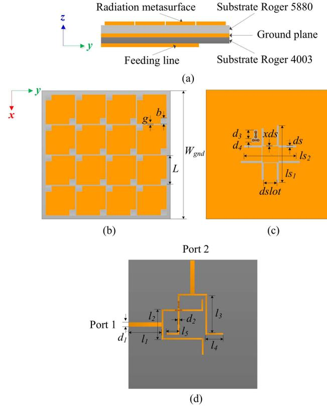
Fig. 6. The geometry of single element antenna: (a) Side view, (b) Radiation metasurface, (c) Ground plane, and (d) Feeding network.
