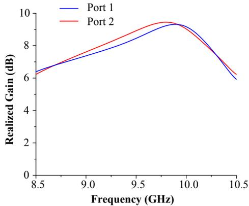
Fig. 9. Simulated gain of proposed antenna.
