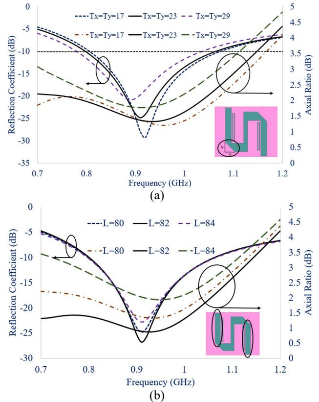
Fig. 2. Parametric analysis in terms of |S11| and Axial Ratio (Dimension in mm)
