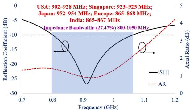
Fig. 4. Simulated  $|S_{11}|$  and Axial Ratio Results.
