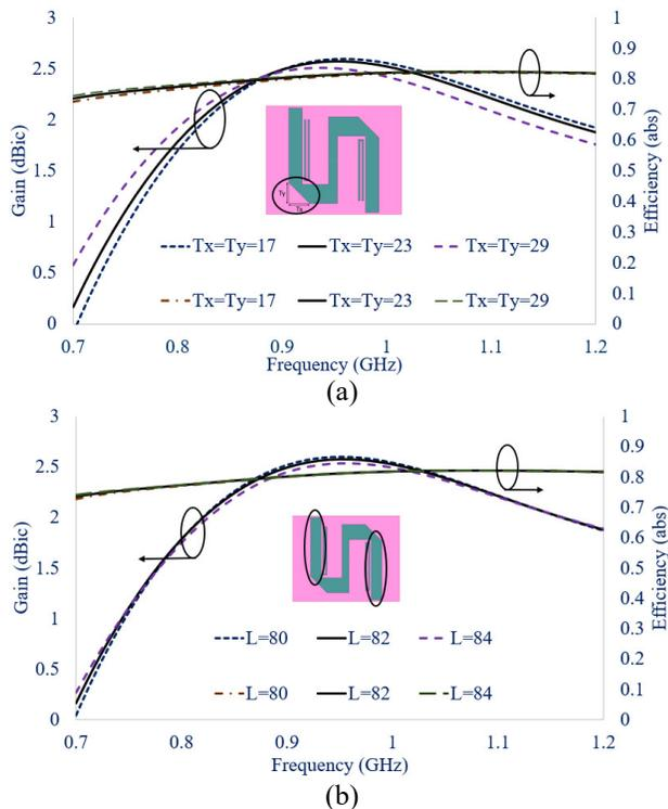
Fig. 3 Parametric analysis in terms of Gain and Radiation efficiency (Dimension in mm)
