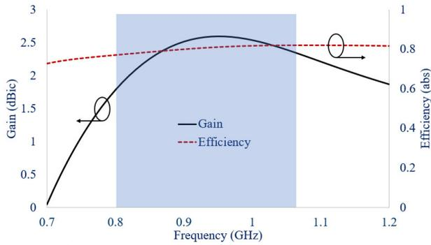
Fig. 7. Simulated Gain and Efficiency Over Frequency.
