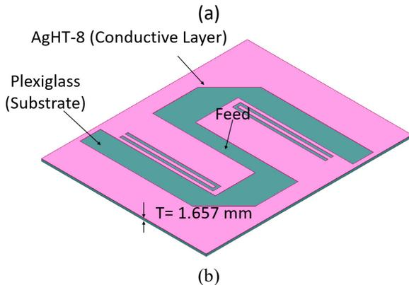
Fig.1 Antenna geometry (a) Top view (b) Perspective view (Dimension in mm)
