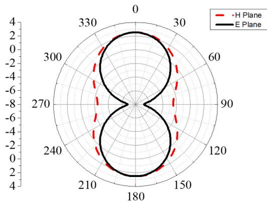
Fig. 5. Simulated radiation pattern at 0.91 GHz in E-plane and H-plane.
