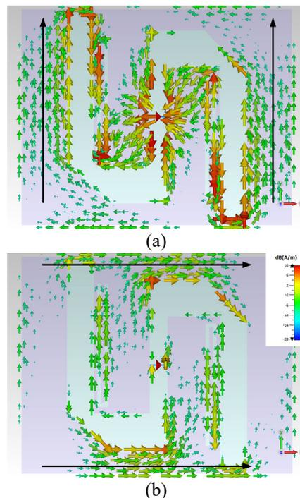
Fig. 6. Surface current distribution of the antenna at 0.91 GHz (a) at  $0^{\circ}$  (b) at  $90^{\circ}$ .
