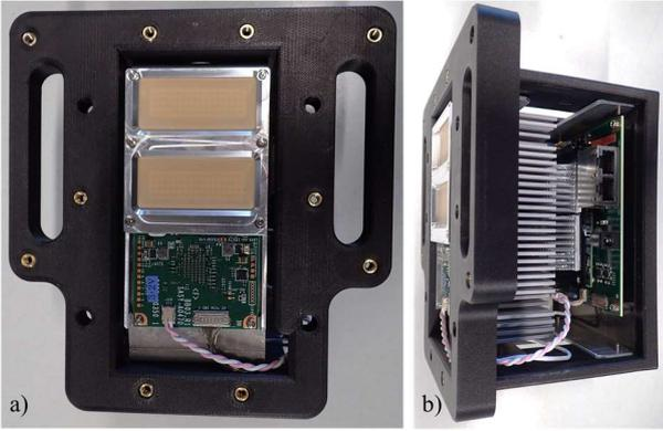
Fig. 10. Fujikura 60GHz mmWave wireless communication module with customized mount. a) front view, b) side view.
